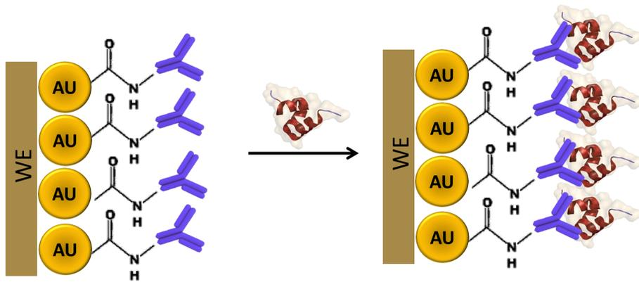
Fig.1: After linking the antibodies to the AuNP using N-Ethylcarbodiimide and N-Hydroxysulfosuccinimide (EDC/NHS), the samples are ready to be measured. The binding of the protein to the antibody on the working electrode (WE) decreases the current, as measured by differential pulse voltammetry.
