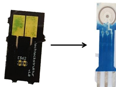
Fig.2: First version of the sensor (left) with a gold surface turning green and a destroyed isolation layer. This happened due to the oxidation of the included copper layer. Therefore we changed to a gold electrode printed on a ceramide surface (right) during development of the protocol
